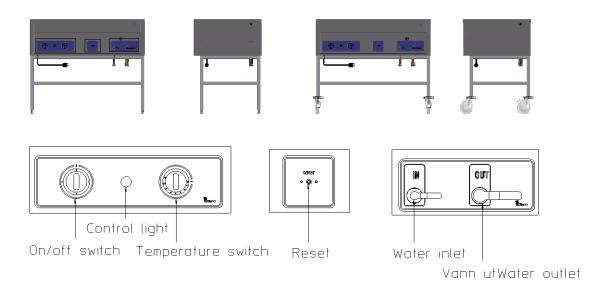
The Bain Marie is made for GN containers hanging on the edge of the well. Different Bain Maries are made for 1/1GN, 2/1GN, 3/1GN or 4/1GN, max. depth of GN containers are 200 mm. It is also possible to use smaller GN containers by using partion bars.
