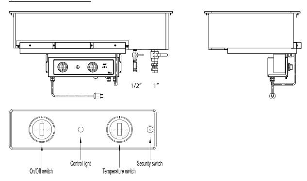
The Bain Marie is made for GN containers hanging on the edge of the well. Different Bain Maries are made for 1/1GN, 2/1GN, 3/1GN or 4/1GN, max. depth of GN containers are 200 mm. It is also possible to use smaller GN containers by using partion bars.
